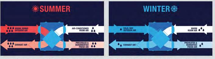
IN SUMMER, THE WARM, HUMID OUTSIDE AIR IS PRECOOLED AND DEHUMIDIFIED BY THE OUTGOING COOL INTERIOR AIR
